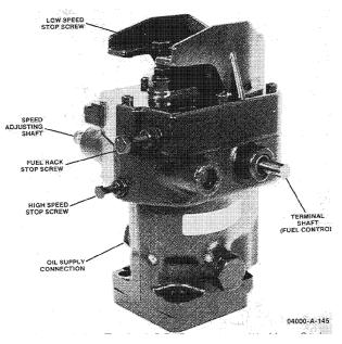
Figure 1-1. Typical SG Governor with New Style Cover
